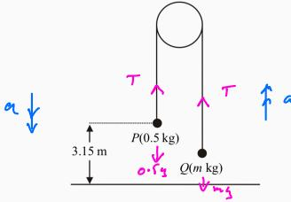
Two particles P and Q have mass 0.5 kg and m kg respectively, where m < 0.5. The particles are connected by a light inextensible string which passes over a smooth, fixed pulley. Initially P is 3.15 m above horizontal ground. The particles are released from rest with the string taut and the hanging parts of the string vertical, as shown in the diagram above. After P has been descending for 1.5 s, it strikes the ground. Particle P reaches the ground before Q has reached the pulley.
